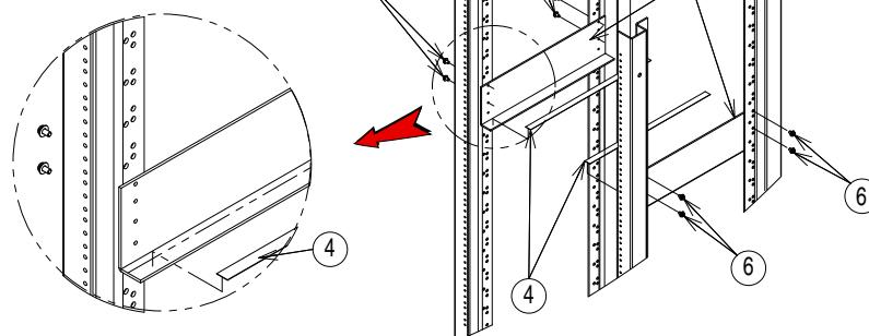
4. Using ⑧ screws and ⑦ washers, mount the instrument in the rack.
