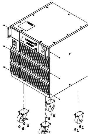
2. As shown in figure, using ③ screws, install ① and ② brackets.
